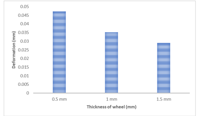
Figure 12: Deformation of wheel with respect to its thickness
