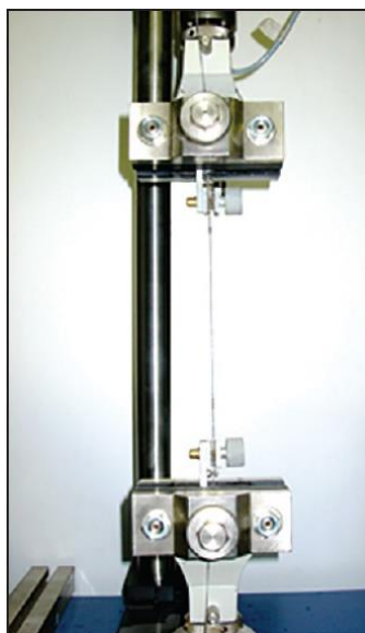
Figure 14. Tensile Testing of Guidewire
