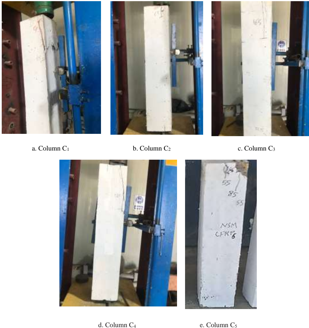
Figure 8. Failure mode of the tested specimens
