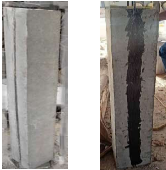
a. Column with groove
