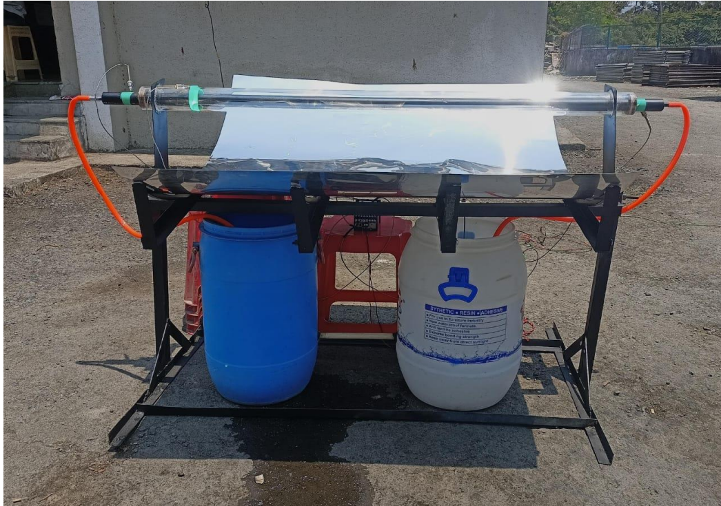
Figure 2. Experimental Setup of Parabolic Trough Collector
