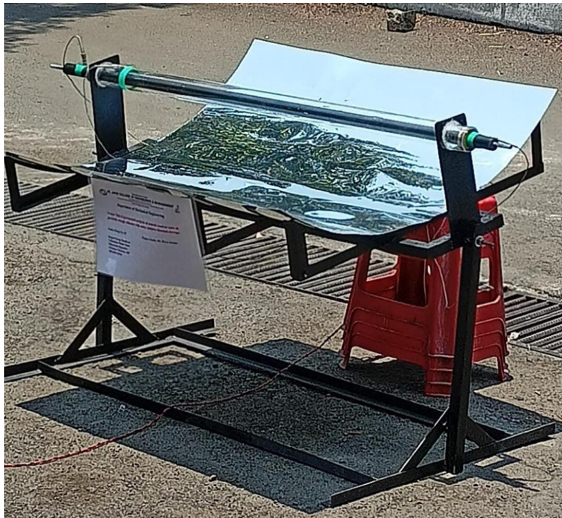
Figure 2. Experimental Setup of Parabolic Trough Collector
