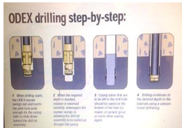
Figure 6. Odex Drilling step-by-step
