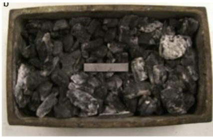
Fig. 1 Pack carburization with stainless steel foil wrapping [5]
