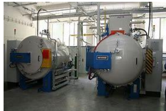
Fig. 2 – Furnaces used for heat treatment hardening experiments: (a) muffle furnace and (b) vacuum furnace.
