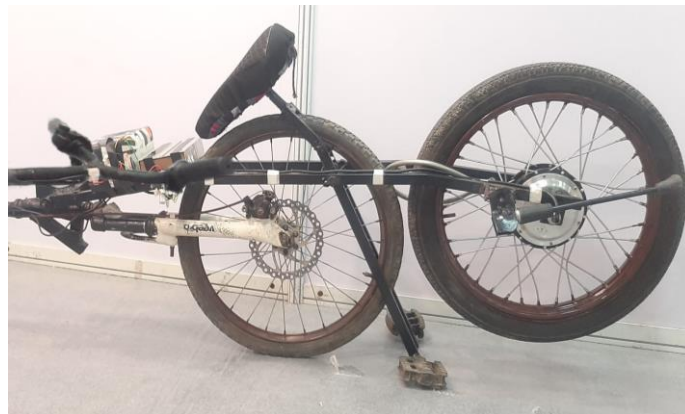
Figure 3. A fabricated model of Electric foldable scooter when it is folded
