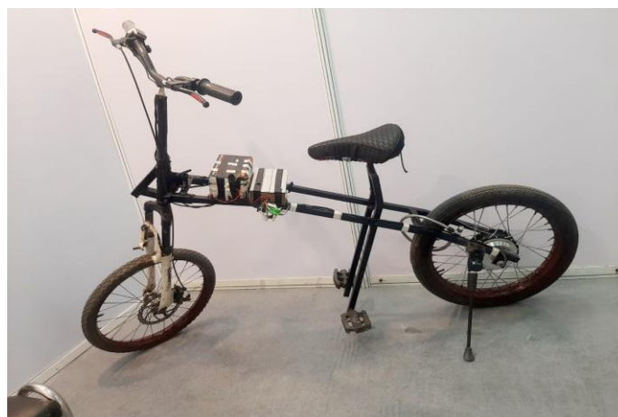
Figure 4. A fabricated model of Electric foldable scooter when it is on stand
