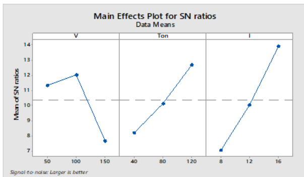
Figure 4: Individual (main) effect plot for S/N ratio (larger-the-better) for AISI 304 material
