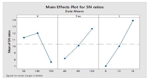
Figure 6. Individual (Main) effect plot for S/N ratio (larger-the-better) for AISI 304 material
