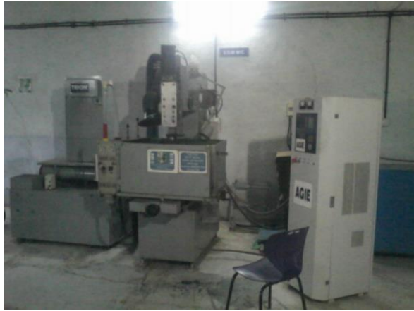
Figure 2. Electric Discharge Machine; model ELECTRONICA-ELECTRA EMS 5535 ZNC (die-sinking type).
