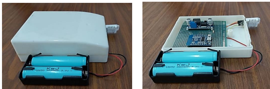
Fig. 8 The physical implementation of the sink node
