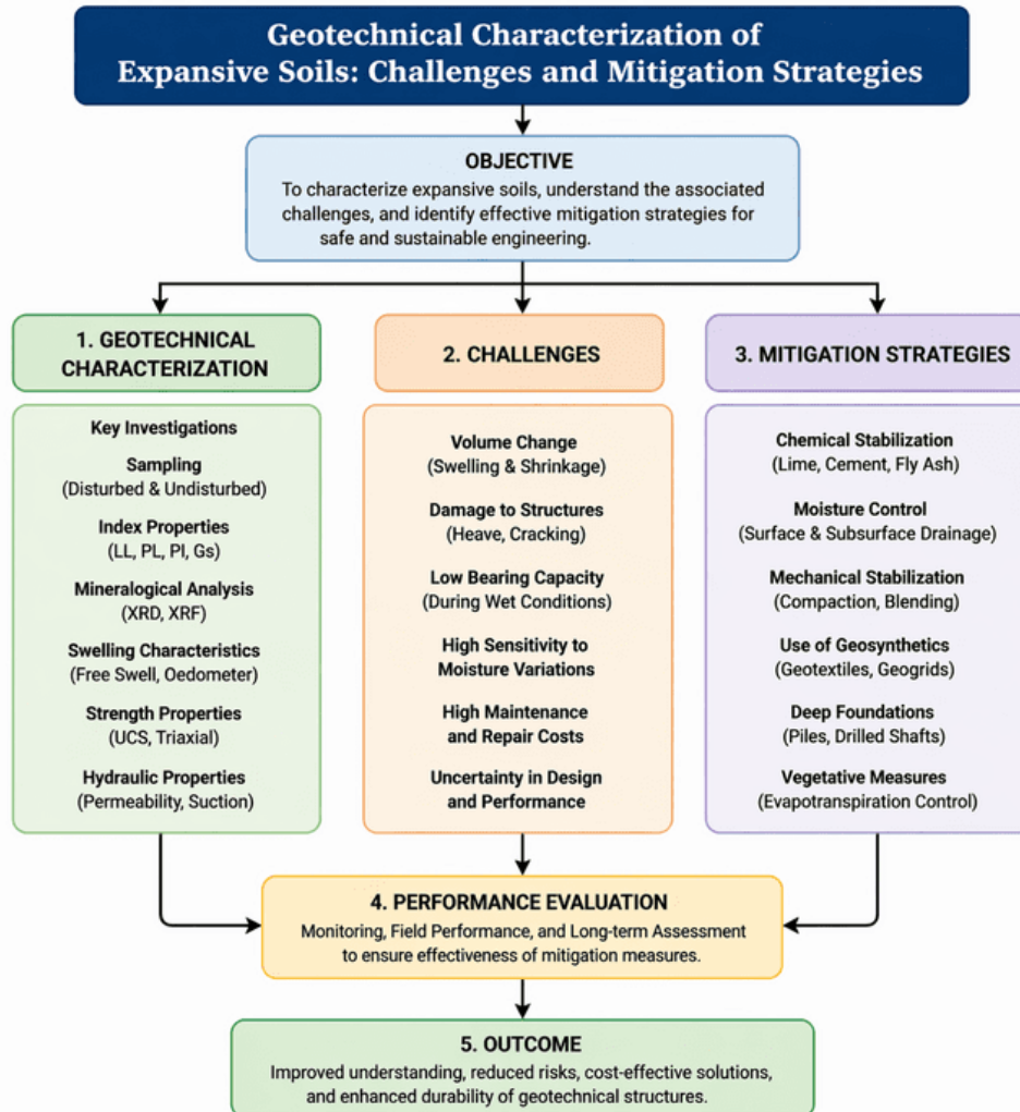
Figure 1. The flowchart of the geotechnical characterization of the expansive soils.
